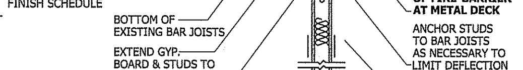
F PARTITION SECTION 1 HOUR FIRE BARRIER U.L. DESIGN NO. U465
