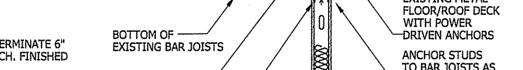
A PARTITION SECTION 3 5/8" METAL STUDS - to bottom of exist. ceiling
